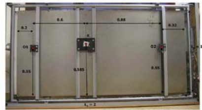
Fig. 1. Exciter (E) and accelerometers (O1 and O2) setup in the stereo EMT140-st unit.
